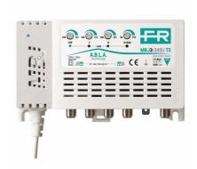
1-input (III+DAB+IV+V) multiband TV indoor amplifier with 35dB gain and up to  $120dB\mu V$  output level on UHF band, separate bands amplification with independent level adjustment (20dB) for each band and low noise figure. T2 technology with UHF cut band for LTE 4G @790MHz and 5G @694MHz.
